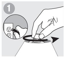
Before beginning **TURN OFF POWER** by unplugging lamp from wall outlet. Unscrew finial and remove lamp shade.
